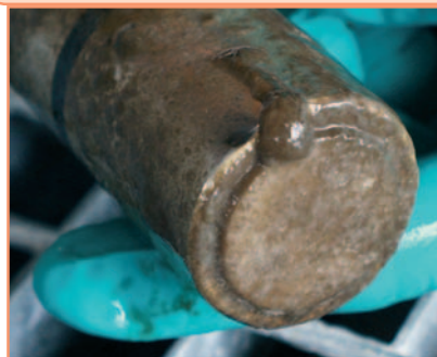
Sensor without ultrasound cleaning system After 16 Days
