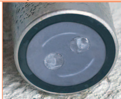
Sensor with ultrasound cleaning system After 16 Days
