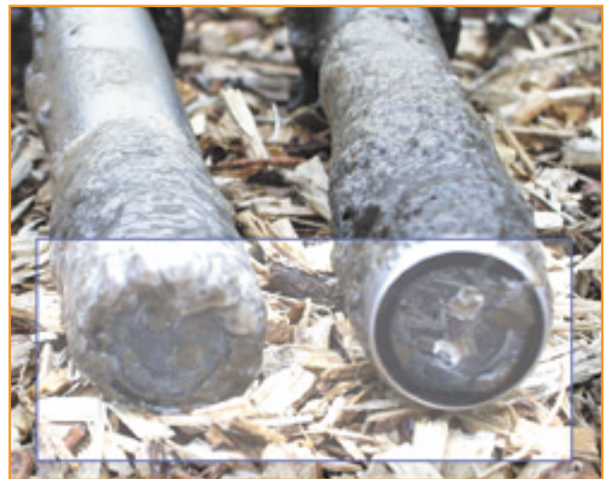
Sensor without and with ultrasound cleaning system
