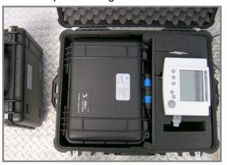
separate and removable case containing rechargeable batteries that provide power supply. A spare battery pack allows for simple on site exchange and uninterrupted field use.
